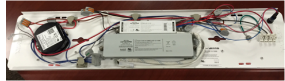
Wiring for 2 foot driver tray
