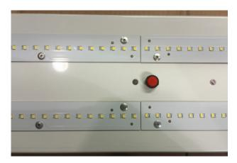
When AC power is applied, the charging indicator is illuminated, indicating that the battery is being charged.
