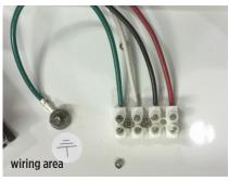
1. Connect power supply leads to terminal block (if supplied) or directly to the black and white driver box.
