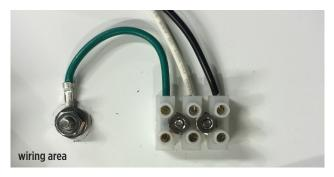
Connect power supply leads to terminal block (if supplied) or directly to the black and white driver box.
