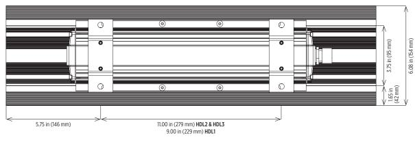
ADJUSTABLE: 1.50 in (38 mm) MIN to 12.50 in (318 mm) MAX
