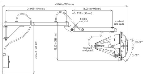
\*indicates maximum adjustment of light beam axis from horizontal
