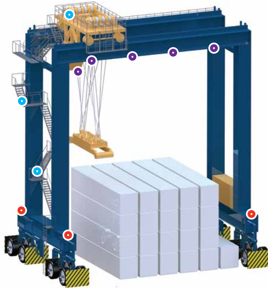
Rubber Tire Gantry Crane
