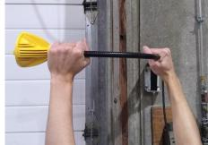
Place one hand near the light head and the other hand near the opposite end of the flexible arm.
