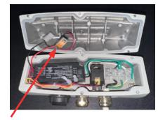
2. Open cover to expose wiring. Disconnect black and red wires going from LED PCB to the lever lock connectors.
