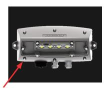
1. Disconnect power to luminaire. Remove front housing cover by loosening the six M6 cover screws. Note that these are captive screws and should not be completely removed from housing cover.
