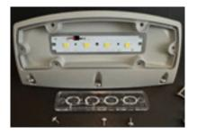
**6.** Ensure new LED PCB is properly aligned with the wires in top left corner. Also make sure optical gasket is flush with housing.
