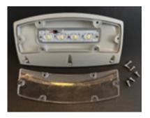
3. Unscrew the six screws securing the lens and remove lens (retain screws). Be careful not to displace lens gasket.
