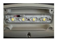
Affix optic properly onto LED PCB and re-tighten the three M3 screws to secure optic. Be sure not to overtighten screws as polycarbonate optic will crack if too much force is applied.
