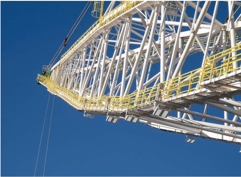
Newly installed ModCom Hi LED fixtures on a boom.
