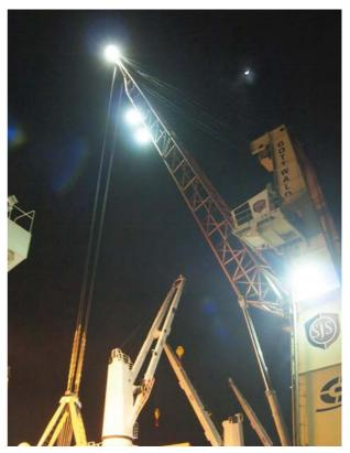
in working position above the hold, light levels indicated up to 46% more lux measured at selected points on the barge and vessel. It was reported by operators that the C.J.L. barge also experiences significantly fewer shadows due to the specified LED optical package.
