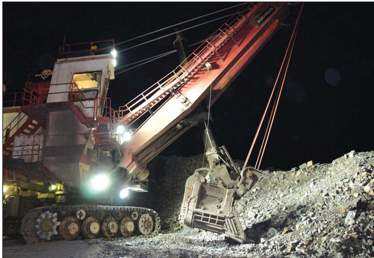
300W Floodlights (Phoenix Products - ModCom® Hi fixtures) on a shovel on an iron ore mine in North America.
