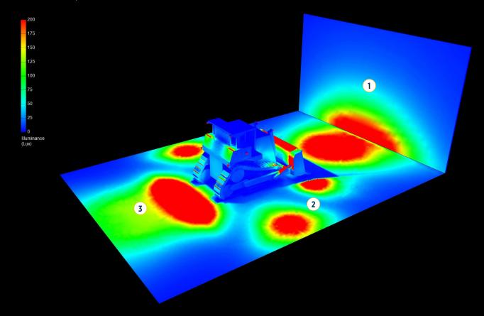
Dozers reverse frequently as they work, making rear lights essential. To aid these maneuvers, some dozers even come installed with rear cameras. To avoid fixture glare on the camera lens – and the operator's vision – use elliptical fixtures that provide smooth, uniform light.
