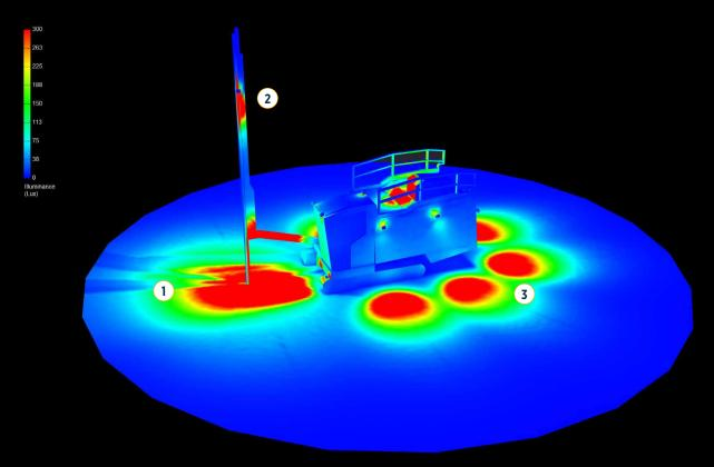
Although blasthole drills are stationary when operating and possess a low top speed, perimeter lighting is still crucial to minimize the threat of accidents or collisions.
