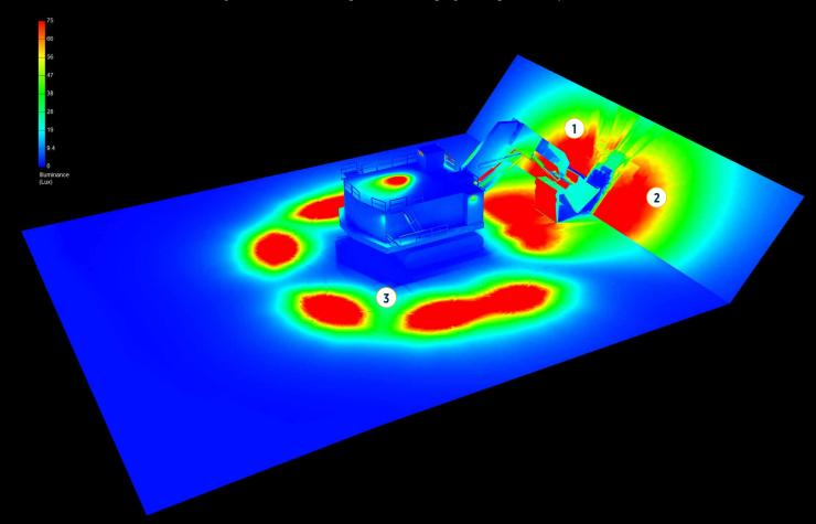
Because hydraulic excavators often work in tandem with haul trucks and wheel loaders, aim to minimize the glare and brightness of their perimeter lighting. Elliptical fixtures – and in some cases flood fixtures – aimed at the ground, work particularly well. This prevents distracting or blinding flashes of light as the excavator turns, thus keeping accidents at bay.
