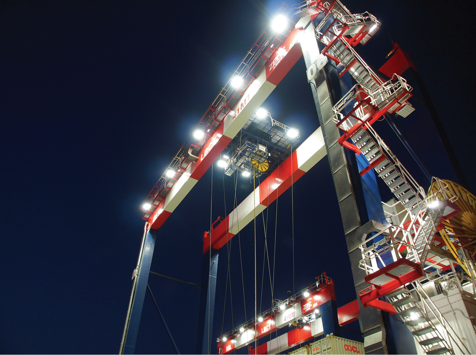
ModCom Hi 300W LED Floodlight illuminating ARMG crane at Long Beach Container Terminal in Los Angeles, CA.
